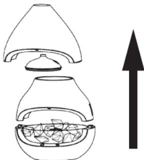
2. Empty the water tank and rinse the tank thoroughly to remove any sediment or dirt. Wipe it dry with a clean cloth or paper towel.
