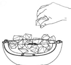
When installing the upper part, please follow the correct direction by matching the grey and round parts of the upper part and the base part as shown in the diagram on the left.
