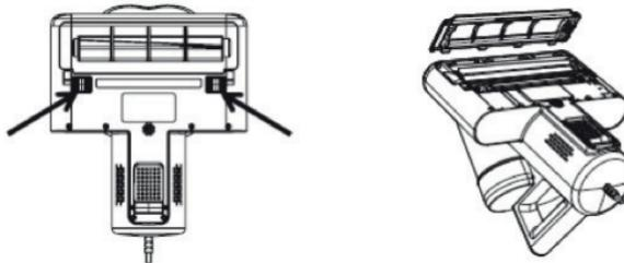
Rinse the roller brush with clean water, dry it thoroughly, then proceed to reinstall.
