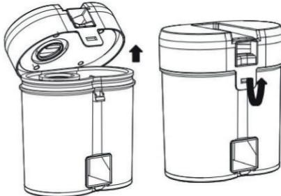
First, remove the stainless steel filter and the HEPA filter from the container. Both filters must be washed with running water, avoiding the use of detergents or abrasive sponges.
