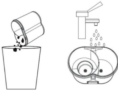
Internal parts must be cleaned separately. Wash each component with water and let it dry completely before reassembling.
